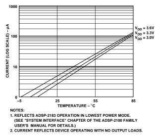
Figure 15. Power-Down Supply Current (Typical)
